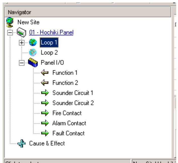
Loop Explorer Panel Configuration for Syncro Lite
