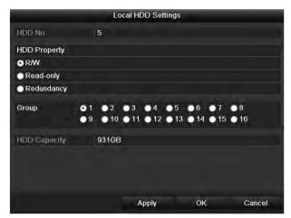
Figure 12. 13 Local HDD Settings Interface
