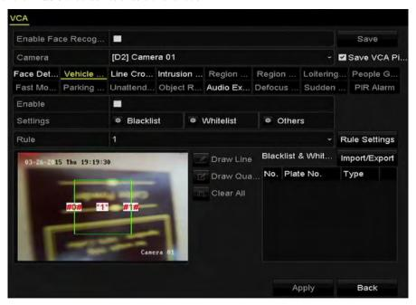
Figure 9. 3 Set Vehicle Detection
