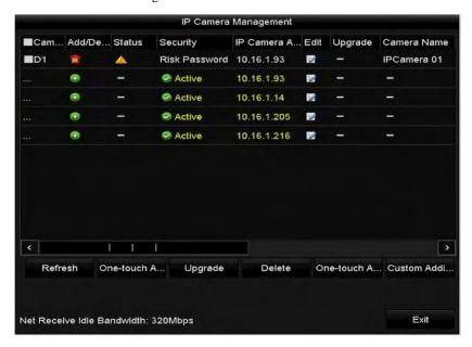
Figure 2. 20 Adding IP Camera Interface
