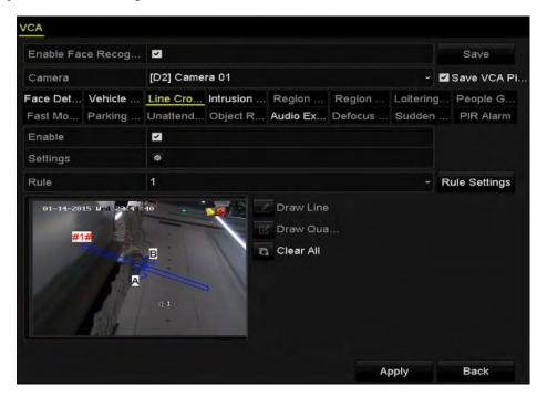
Figure 9. 6 Draw Line for Line Crossing Detection
